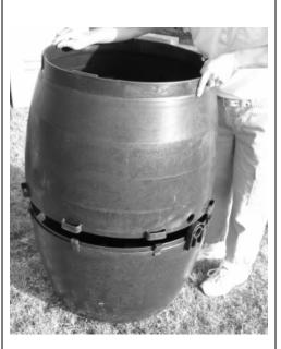
The barrel halves use a tongue & groove connection. Be sure to coat the tongue (lip) on the bottom half of the barrel with vegetable oil, soap, or Vaseline, otherwise assembly will be much more difficult. Align the barrel halves as shown here on the left. Align and insert each latch as seen here on the right and then work the tongue & groove together so it is securely seated all the way around the barrel. This may take working around the unit several times for it to seat properly.
