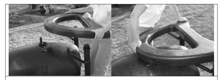
Align the second Stand Half with the Pivot Rod, both Gusset Braces, and both Stand Supports. At first, gently align all of these parts with the appropriate holes being careful not to damage the Retainer Rings. Just let the Stand Half rest in place. Then by hand, press the Retainer Rings up into place over the Stand sockets. Now firmly press down on the Stand making sure all of the components are inserted with their locks fully engaged.
